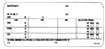
This sticker is located on the driver's door pillar and signifies our compliance with the Federal Motor Vehicle Safety Regulations. This sticker lists the date the van was manufactured, the serial number of the van, the gross vehicle weight rating, tire and rim size and recommended tire pressure.
